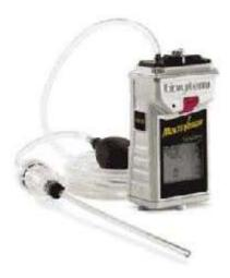
This is an example of a confined space gas meter. This unit has a probe attachment which can be lowered down into a confined space for remote readings.
